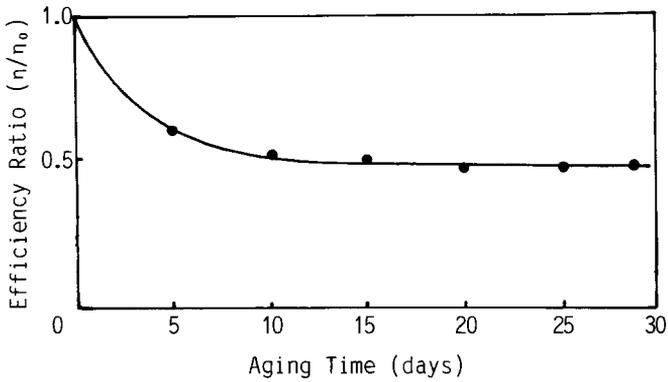
Fig.8 Aging of the conversion efficiency of the solar cell in argon environment.
