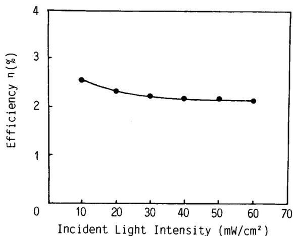
Fig.5 The dependence of the conversion efficiency of  $\text{Al}/[\text{CH1y}]_x/\text{Au}$  solar cell on incident light intensity.
