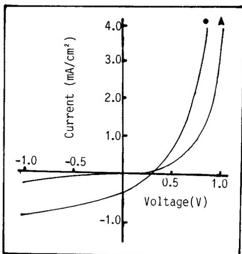
Fig.1 The J-V characteristics of Al/cis-[CHI<sub>y</sub>]<sub>x</sub>/Au solar cell
