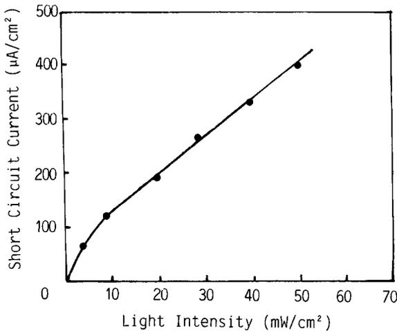
Fig.4 The dependence of the short-circuit current of  $Al/[CHI_y]_x/Au$  solar cell on incident light intensity.
