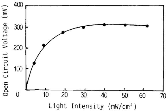
Fig.3 The dependence of the open-circuit voltage of  $Al/[CHI_y]_x/Au$  solar cell on incident light intensity.
