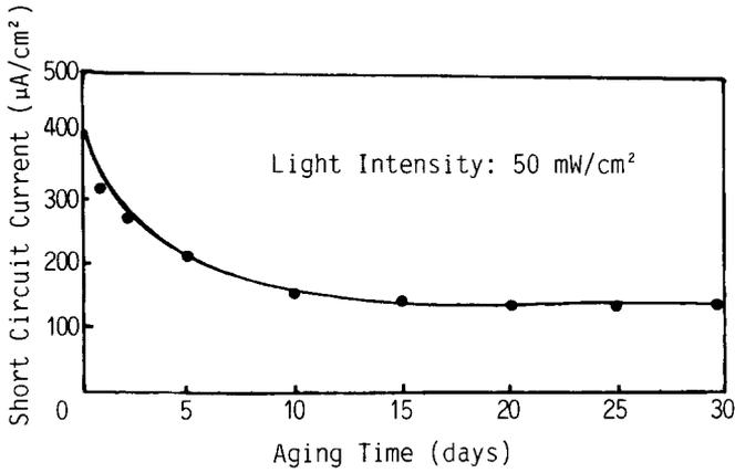
Fig.7 Aging of the short-circuit current of the solar cell in argon environment.
