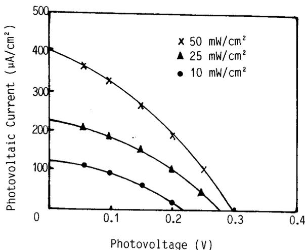
Fig.2 The photovoltaic properties of Al/[CHI<sub>y</sub>]<sub>x</sub>/Au solar cell under various illuminations.
