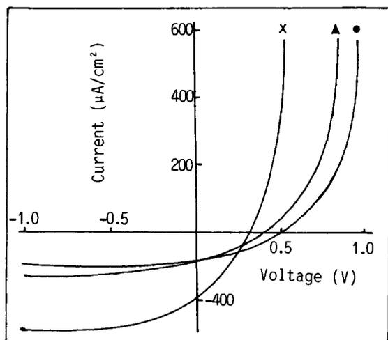
Fig.6 The J-V characteristics of  $\text{Al}/[\text{CH1y}]_x/\text{Au}$  solar cell in argon environment under illumination of light intensity of 50  $\text{mW}/\text{cm}^2$ .
